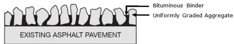
Cross-section of a one-size seal coat aggregate
